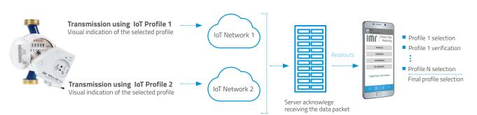
Check communication and select appropriate IoT profile that ensures stable APULSE reception. Available IoT Networks: LoRa, Sigfox.
